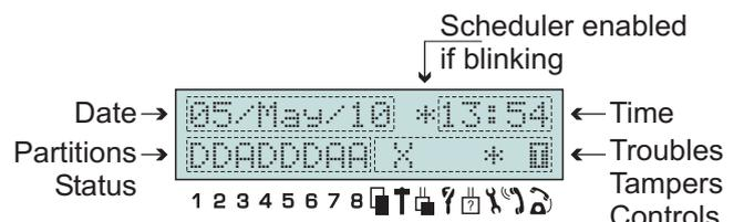
**Figure 3** The display of a LCD keypad during View partition status (MAIN PAGE).
